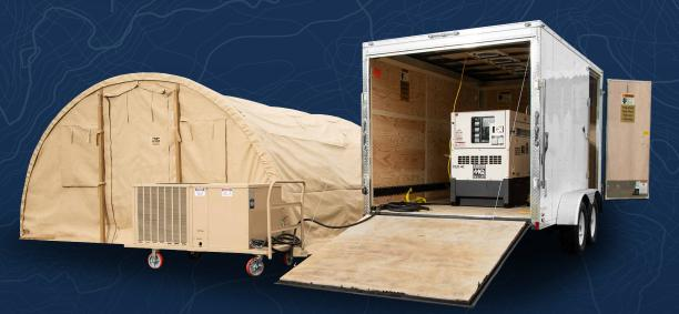
CAMSS Shelters has added a new essential item to their product line. Introducing the Medical Trailer. When accessibility is limited, you can count on CAMSS Shelters Medical Cargo Trailer. Most commonly used on and off the field for rapid medical emergencies. This portable packaged includes a 2.5 Ton ECU, 14kW Generator and a 16QE shelter.
